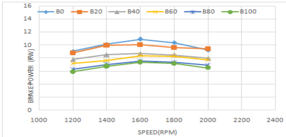
Fig.4. Variation of brake power with engine speed for standard diesel and biodiesel blends
